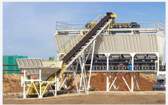
Shuttle Type Automated Aggregate Feeding System
