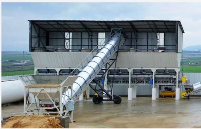
Radial Type Automated Aggregate Feeding System
