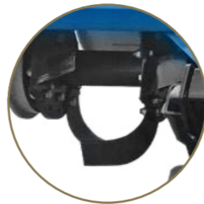
Hydraulic sliding system ensuring safety for trees
