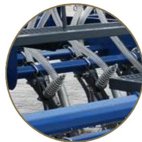
Spring tines offers machine safety
