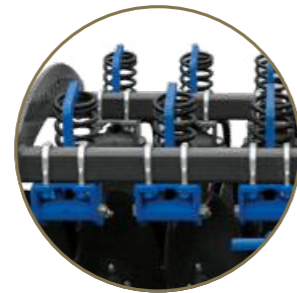
Uninterrupted tillage with independent springs
