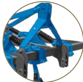
Breaks the hardened base inside soil
